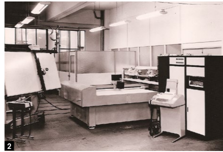
1 Company founder Junzo Kashiya 2 Grading machine modifies and cuts basic sewing patterns
